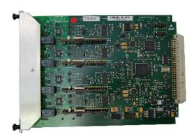
The Telephone Expansion Board (FXO) is one of the option cards available for the Gemini™ Intercom system.
