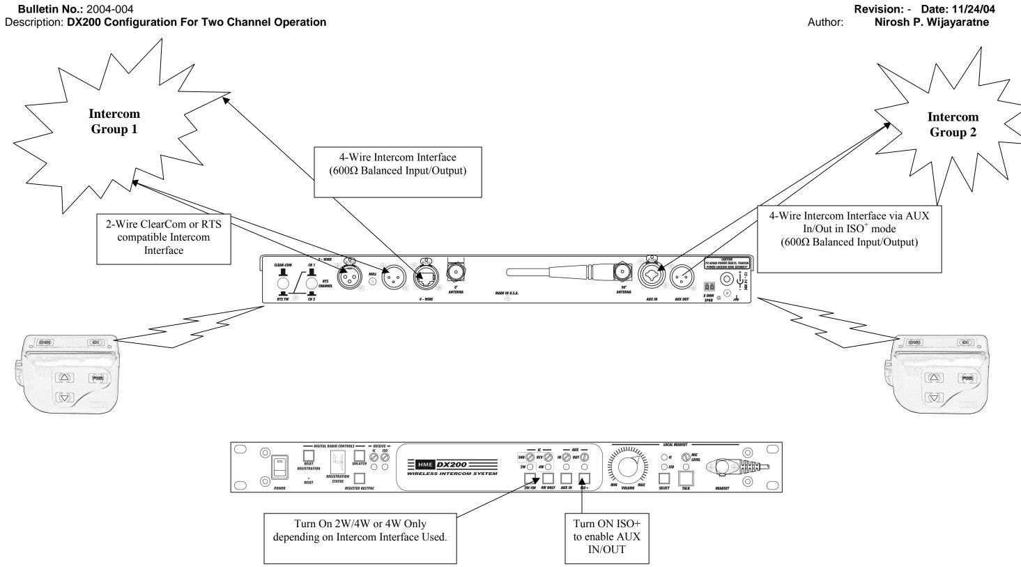
Press IC button to talk to **all beltpac users** plus wired users connected through 4-Wire RJ45 or ClearCom/RTS interfaces Press ISO button to talk to **all beltpac users** plus wired users connected through AUX IN/OUT interface.
