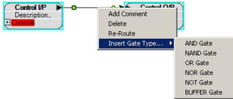
Figure 1-76: Inserting a Logic Element into a Connection
