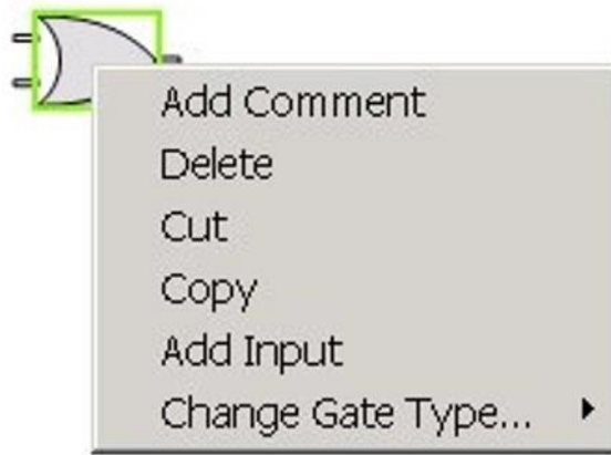
Figure 1-79: Menu Options for OR Logic Element
