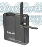
FreeSpeak Edge™ is a member of Clear-Com's FreeSpeak™ family of digital wireless intercom solutions. A FreeSpeak Edge IP transceiver forms a link between FS Edge 5GHz beltpacks and a Clear-Com matrix (E-IPA-HX interface card). The transceiver is designed for use on AES67 enabled Local Area networks (LAN). It requires careful setup of an AES67 compatible network switch with PTP. For details see: Clear-Com AoIP network and switch recommendations.
