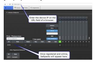
Note: The IP address allocation is set to Dynamic Host Control Protocol (DHCP) as default.
