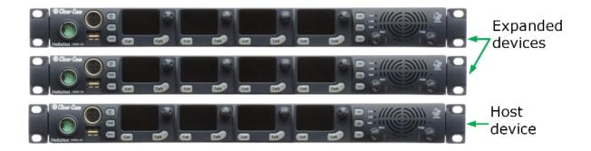
Multiple HelixNet Remote Stations can be joined together in an expansion mode for additional channels. To set up an expansion group, once the devices have been connected to the same LAN by Ethernet cable, you will need to identify a **Host** device. This is done from the front panel menu of the device under **Networking**. Then designate the panel(s) to be stacked as expansion panel(s).
