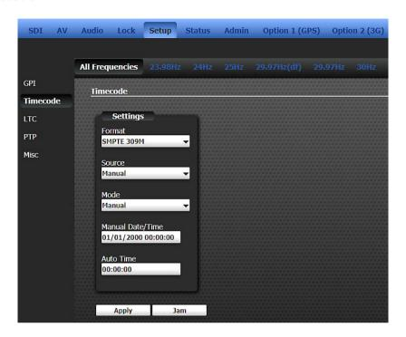
Four timecode formats are supported from the format menu: the chosen format applies to all timecode generated by the Mentor RG. The different format options place date/time data into the binary groups of the VITC/LTC codeword in a different sequence. See the table (below) for more detail.
