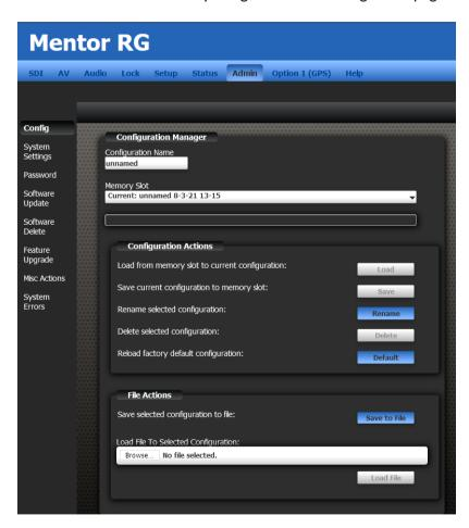
The "Configurations" dropdown list allows the selection of either the current (active) memory or one of the four memory slots.
