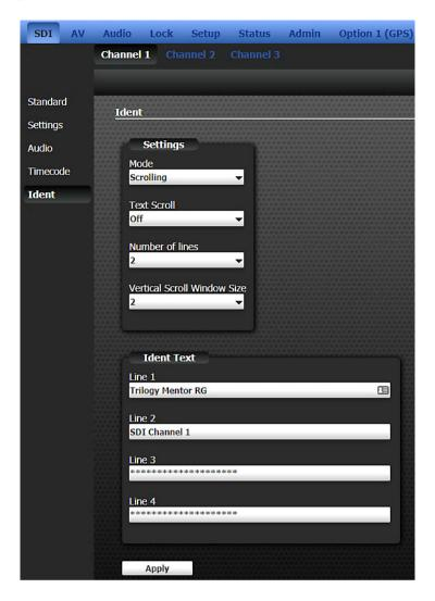
Using the ident menu, choose the "Number of Lines" of text before entering text using the "Ident Text" fields. Lines that are not available are indicated by a string of asterisks.
