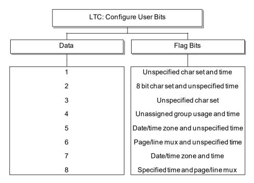
The primary function of the User Bits is to allow the operator to embed a date code within the data stream since timecode represents only embedded time. This conforms to SMPTE S309.
