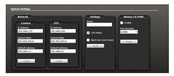
Mentor RG network settings can be changed here: remember that if you change the network address to a different subnet, you may lose contact from your current PC address.
