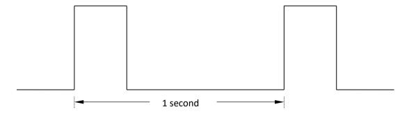
The leading edge of the positive going pulse provides the timing reference plane for locking external equipment. There is no agreed standard for the pulse width.
