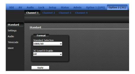
The table in section 17.2 shows the available standards. This page includes the option to enable/disable 3G Level B.
