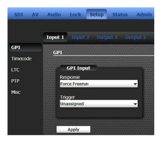
When a GPI input is asserted, it can cause one of a number of responses. The menus also provide choice of the trigger point, e.g. rising or falling edge. Choices of Response and Trigger are shown below.
