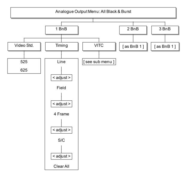
*Note 1*: VITC menu branch is only displayed when the Timecode software feature is enabled.
