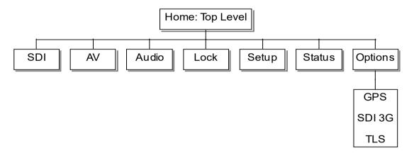
As explained above, this is a typical arrangement although others are possible. Further information on the menus for each option board are given in the following chapters.
