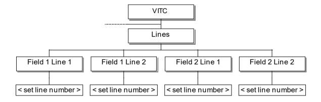
Here, "Line1" or "Line 2" indicates the first and second lines in each Field that have VITC inserted.
