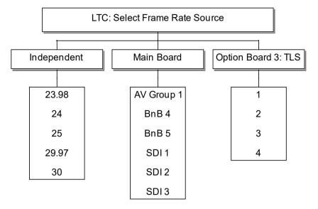
Since LTC is not contained within a video waveform, the timing must either be set explicitly or allied to one of the signal outputs.
