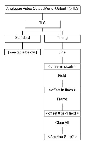
Note: the option for Timing at Field level is only displayed for "interlaced" video standards, not for "progressive" standards.
