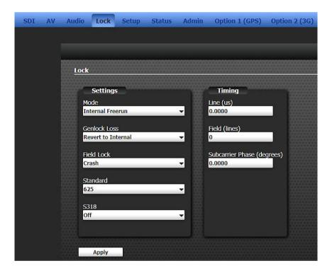
The Genlock (or Generator Lock) settings of the unit (for example, the current Genlock mode and timing offsets) may be changed as follows:
