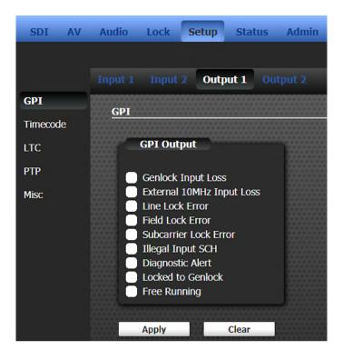
The image above shows the events which can be used to "fire" GPI output 1: GPI output 2 is independent but configured in precisely the same manner. Any number of events may be checked, they will act as a logical "OR".
