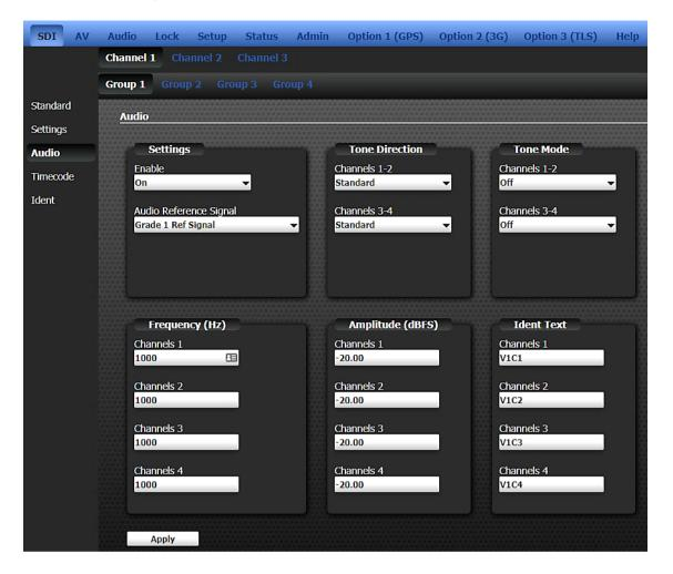
Four simultaneous AES Groups are available from both the mainboard outputs and the 360-20-00 HD/3G-SDI option board if fitted.
