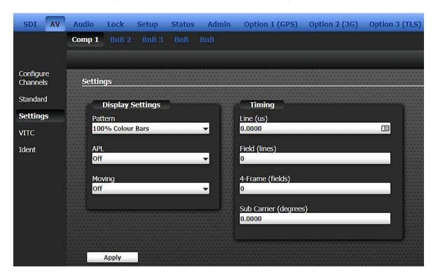
The range of available patterns depends on both the line standard selected and the output configuration (composite, YUV etc.).
