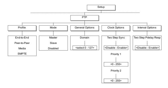
The front panel menus offer a limited selection of the available settings, as shown above. The full range of parameter settings is provided via the Vector web interface.
