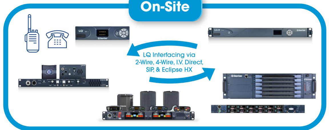
Hybrid Intercom using Gen-IC Premium LQ Interfacing
